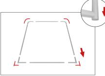
Step 5: Push banner stand frame onto posts of flat base or optional feet. Press evenly on both sides to make easier for the frame to go on.
